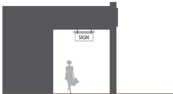
FIGURE 12-6: SUSPENDED PEDESTRIAN SIGN
